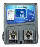
**CHYT0444AU:** pH and ORP controller automatically controls your sanitiser and pH levels via two onboard DULCOFLEX peristaltic pumps that dose your liquid sanitiser and diluted acid. The Odi Touch is a versatile and multi-parameter monitoring and dosing System, offering up to 8 parameters for precise water analysis. It provides options for monitoring free or active chlorine, total chlorine, pH, conductivity, temperature, and more.
